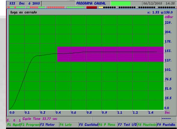
Leak test real time graphics.
