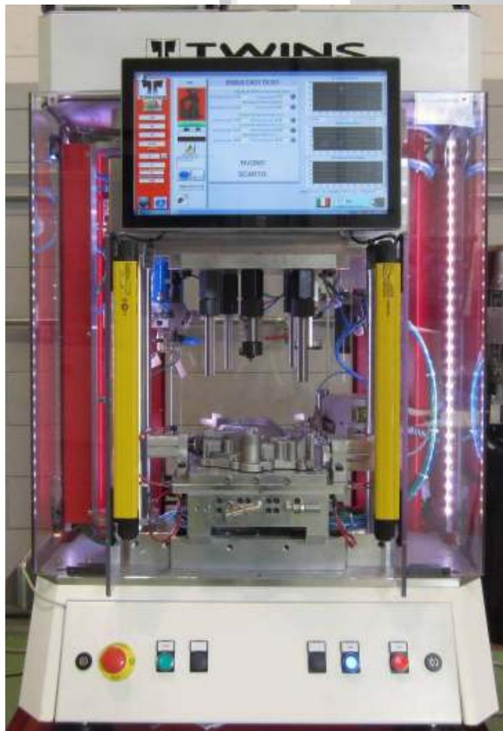
Leak testing machine with pallet, suitable for:
