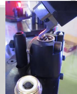
Spindle CNC inserting in the body Ball loading with preventing shock inserting.
