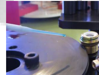
Loctite dispensing all around the fitting Gaskets automatic loading and orienteering.
