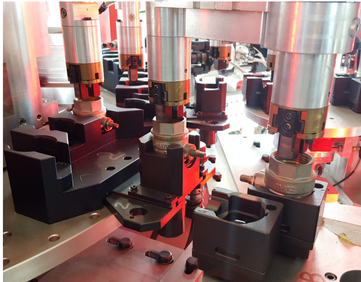
CNC leak and polymerization system, using the main disk. High reliability and high precision, leak rate until 20cc/h
